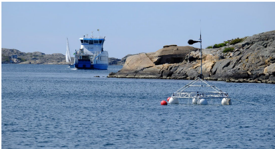
Figure 1. Simultaneous measurement of airborne and underwater noise as well as onboard vibrations of the Styröbolaget ship “Elvy”, May 2022.
